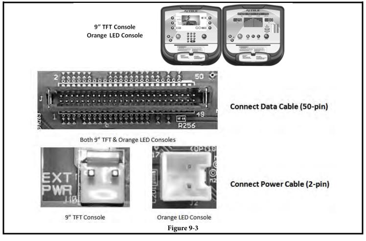
**NOTE:** Ethernet & Coaxial cable connections are not available on the Orange LED or 9" TFT Consoles **All Ground Wires Must be connected**
